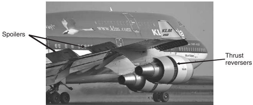
Figure 8.17 Thrust reverser and ground spoiler deployment
